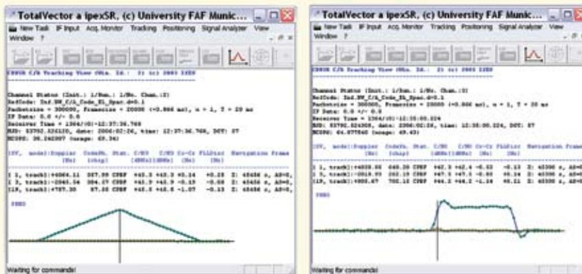
FIGURE 6 Comparison of standard (left) and waveform (right) multi-correlator
